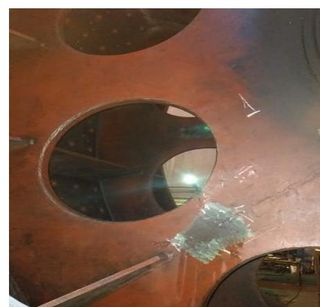
Fig. 2. Fragment of the butt welded joint of the rotor rim disks
