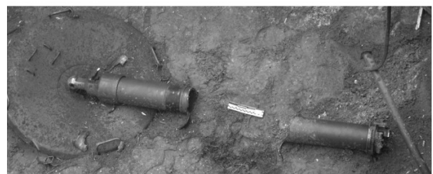
Fig. 1. A mortar barrel rupture
