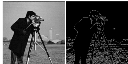
Fig. 4. Grey scale image and applied edge detection filter image [1]
