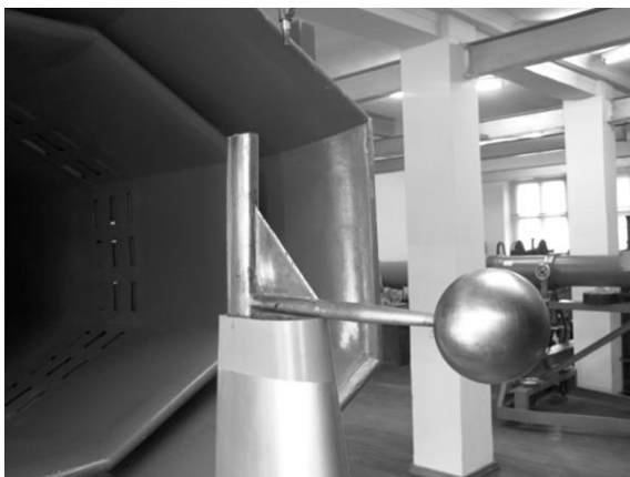
Fig. 9. Drained metal sphere in the working part of the subsonic wind tunnel T-1
