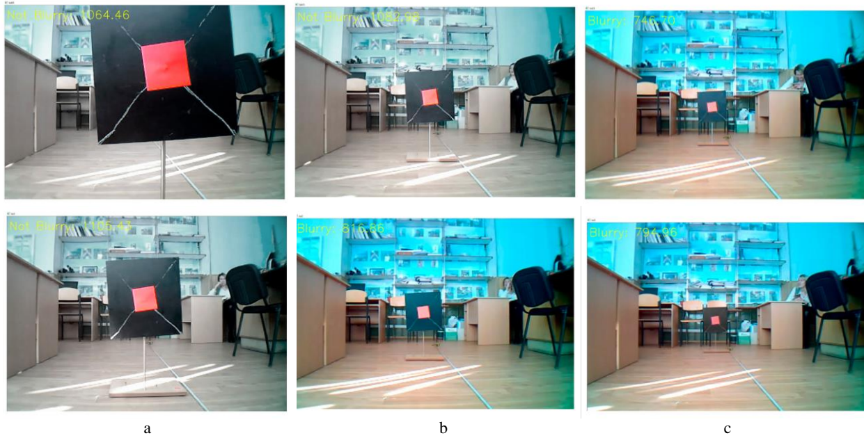
Fig. 1 Set of images for determining the blur depending on the distance: a – is the distance 0.5 and 1m; b – is the distance 1.5 and 2m; c – is the distance 2.5 and 3m
