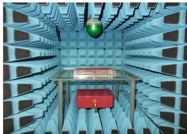
**Fig. 7.** Small microwave chamber used in biomedical research
