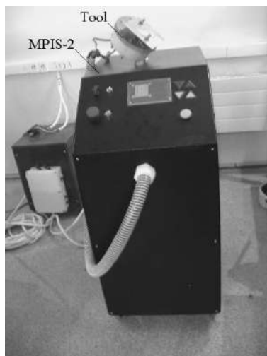
Fig. 5 – The magnetic-pulsed installation MPIS-2 with a tool, (maximum of the stored energy is \sim 2,4 kJ at voltage \sim 2 kV)
