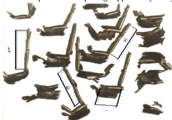
Fig. 2 – Chips cut by the finishing cutter ( m=20 mm) without teeth cutting by a cutter with a prominence
