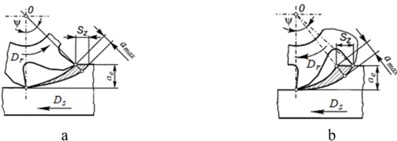
Figure 1 - Cutting patterns for up (a) and down (b) end-milling [10] a_e – radial cutting depth; a_{max} – maximum thickness of the layer to be cut; S_z – feed per tooth
