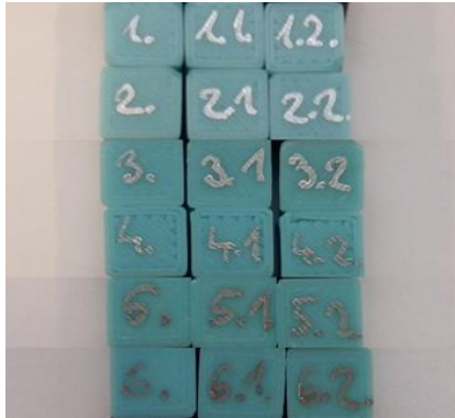
Figure 3 – 3D printed ABS samples for compression test
