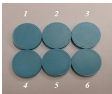
Figure 1 – 3D printed ABS samples for ball-on-disk test
