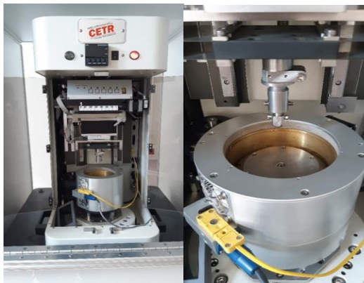
Figure 4 – CETR – UNMT1 Universal Micro-Nano Materials Tester
