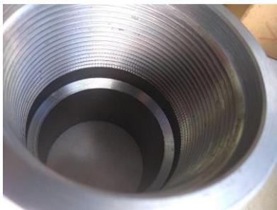
Figure 1 – Part with notches on the thread
