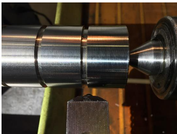
Figure 3 – The technological realization of sliding burnishing process
