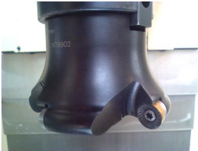
Figure 1 – The applied milling head with one round insert
