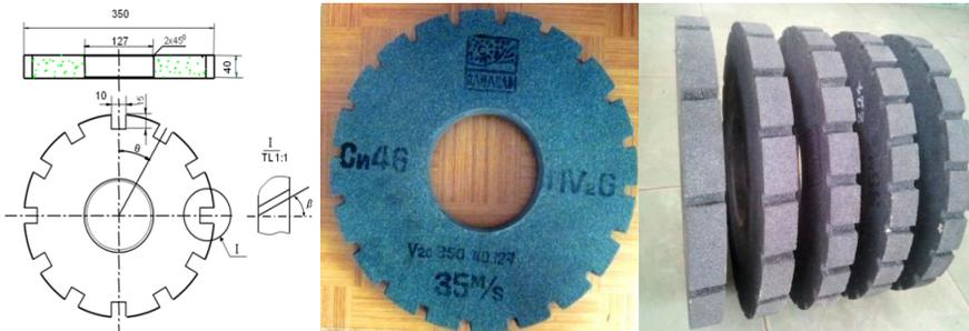
Figure 1 – Geometry parameter of segmented grinding wheel with angle  $\beta$  slot's width  $w$  and slot's depth  $b$
