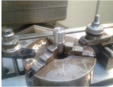
Figure 4 – Clamping of the machined specimen
