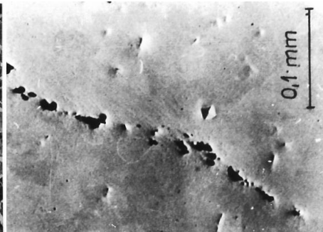
Figure 3 – A typical rigid Al_2O_3 inclusion of steel over-deoxidized with Al
