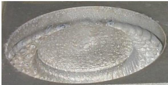
Figure 2 – Milling with Abrasive Waterjet
