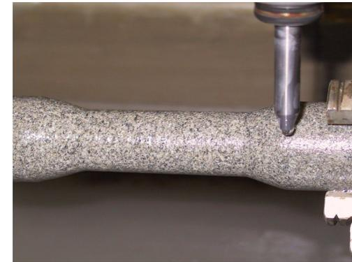
Figure 3 – Turning with Waterjet
