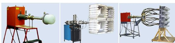
Fig. 5. Compact powerful ultra-wideband sources of radiation with capacity up to 1 GW developed at Tomsc Institute of High Current Electronics
