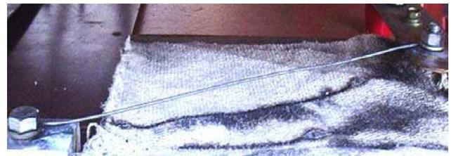
Fig. 2. General view of a round galvanized steel wire ( $r_0=0.8$  mm;  $l_0=320$  mm;  $\Delta_0=5$   $\mu$ m;  $S_0=2.01$  mm<sup>2</sup>) placed in air above a heat-shielding asbestos cloth and rigidly fixed in the discharge circuit of the PCG-C generator ( $W_C \approx 310$  kJ;  $U_C \approx -3.7$  kV before an aperiodic current pulse of high density flows through it [9])
