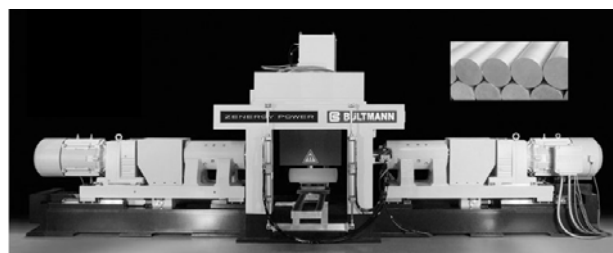
Fig. 3. Induction heating of billet rotating in superconducting system (Weseralu, Germany, 2009)
