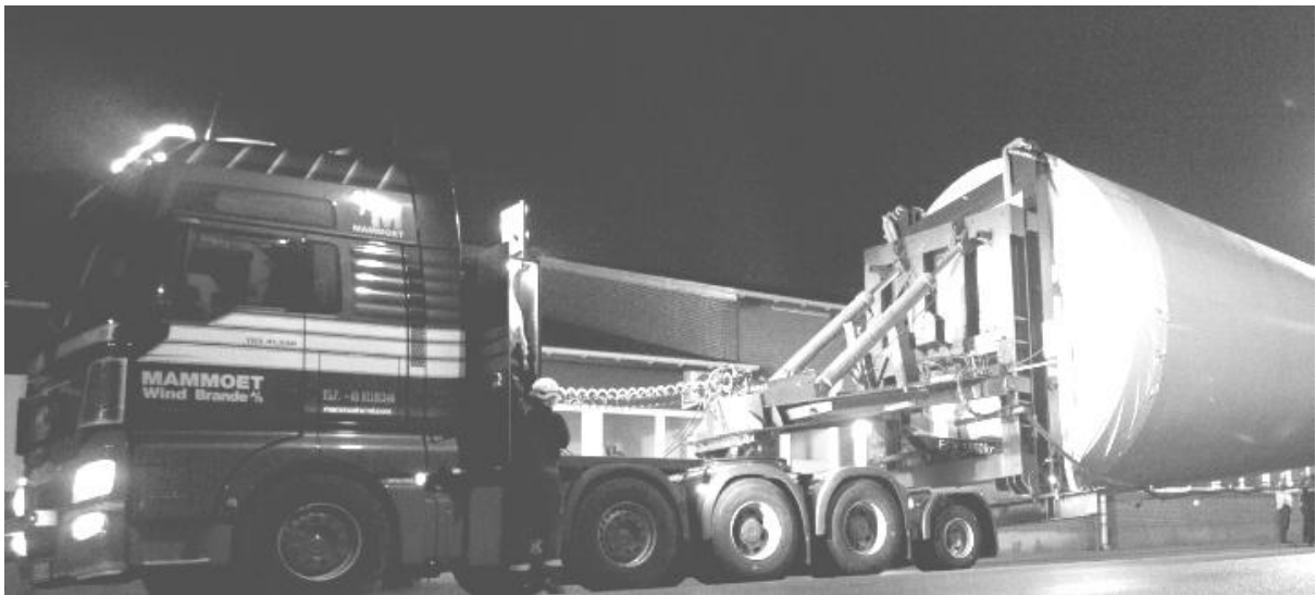
Figure 3 – Transporting the blade with a length of 80 m using a universal adapter (red construction)
