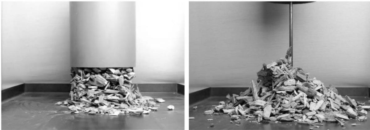
Figure 3 – Angle of repose test with cylinder (250 mm diameter)
