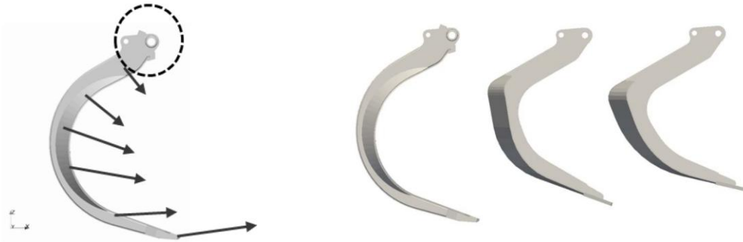
Figure 11 – Movement profile of the grab shell
