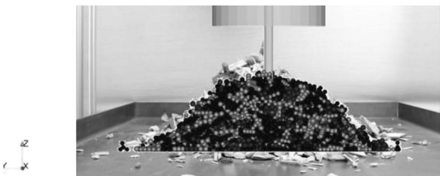
Figure 7 – Calibration of the angle of repose in simulation and experiment
