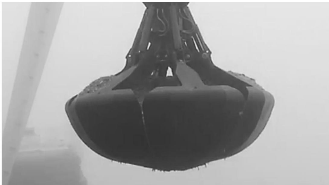
Figure 14 – Fully closed grab with optimized shells when unloading a ship
