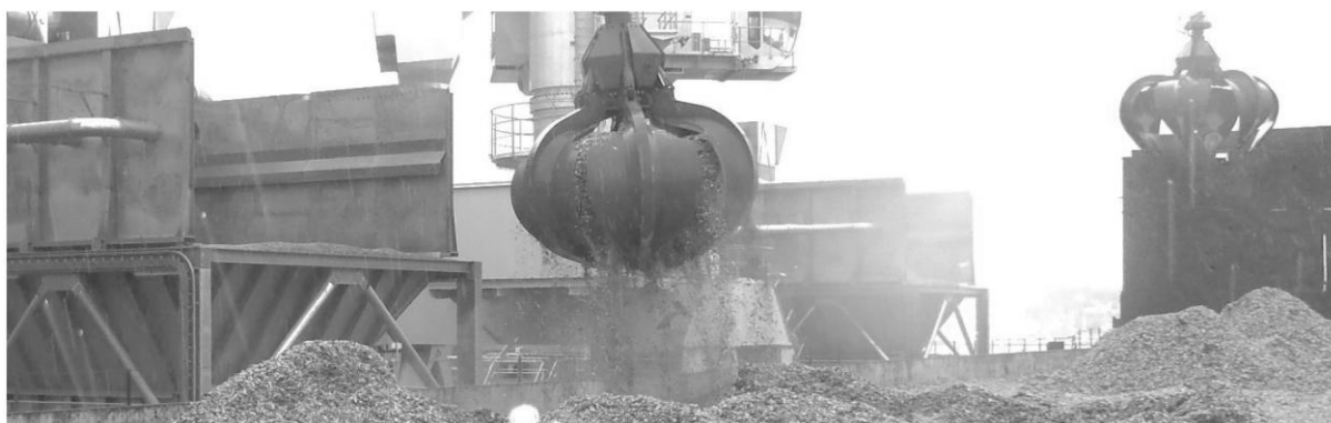
Figure 1 – Conventional orange peel grab with partially closed shells during ship unloading of wood chips
